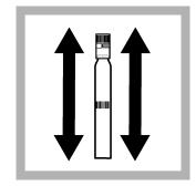
**4.** Shake the vial 2–3 times to dissolve the reagent in the cap.
