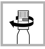
**3.** Turn the DosiCap Zip over so that the reagent side goes on the test vial. Tighten the cap on the vial.
