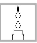
2. Use a pipet to add 0.2 mL of sample to the test vial. Immediately continue to the next step.
