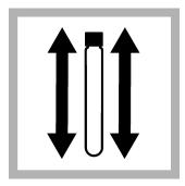
13. Put the caps on both vials. Shake vigorously for 15 seconds to mix. The reagent will not dissolve completely. Undissolved powder will not affect the accuracy of the test. The solution will start to turn yellow.
