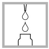
4. Prepare the blank: Add 0.5 mL of deionized water (included in the kit) to the second vial.
