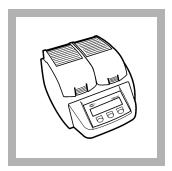
**1.** Start the DRB200 Reactor. Set the temperature to 105 °C.
