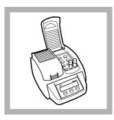
**6.** Put the vials in the reactor and close the lid. Leave the vials in the reactor for exactly 30 minutes.
