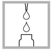
**15. Prepared sample:** When the timer expires, use a pipet to put 2 mL of the digested, treated prepared **sample** into one TN Reagent C vial.
