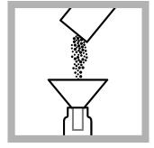
2. Use a funnel to add the contents of one Total Nitrogen Persulfate Reagent Powder Pillow to each of two HR Total Nitrogen Hydroxide Digestion Reagent vials. Make sure to clean any reagent that gets on the lip of the vials or on the vial threads.
