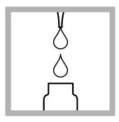
**16. Blank:** When the timer expires, use a pipet to put 2 mL of the digested, treated **blank** into the second TN Reagent C vial.
