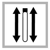
5. Put the caps on both vials. Shake vigorously for at least 30 seconds to mix. Undissolved powder will not affect the accuracy of the test.
