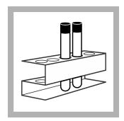
7. At 30 minutes, use finger cots to immediately remove the vials from the reactor. Let the vials cool to room temperature.
