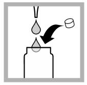
1.3 mL of Solution A and 1 Reagent B tablet in quick succession to a dry 20-mm reaction tube. Close the reaction tube
