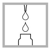
**8.** Use a pipet to add 0.2 mL of Solution D to the test vial
