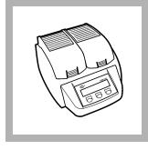
**11.** Close the reactor. Let the vials react for 2 hours at 103 to 105  $^{\circ}$ C.
