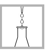
**3.** Add 0.4 mL of Buffer Solution to the Erlenmeyer flask, pH 2.0. Use pH paper to make sure that the sample pH is 2.
