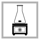
**4.** Put the flask on a stir plate. Stir at a moderate speed for 10 minutes.
