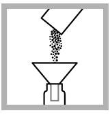
5. Put a label that says "Reagent Blank" on one Low Range Acid Digestion vial. Put a lable that says "Sample" on a second Low Range Acid Digestion vial. Add the contents of one TOC Persulfate Powder Pillow to each Acid Digestion Vial.
