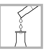
2. Add 10 mL of sample to a 50-mL Erlenmeyer flask. Put the stir bar in the Erlenmeyer flask.
