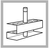
**12.** After two hours, remove the vials from the reactor. Put them in a test tube rack to cool for one hour. Make sure that the vials stay in an upright position at all times. The liquid in the blank should show a dark blue color.
