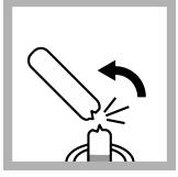
9. Put one unopened ampule into each Acid Digestion Vial. Snap the top off of the ampule when the score aligns with the top of the vial. Let the ampules drop into the vials. Do not invert or tilt the vials after the ampule is inside.
