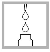
**7. Prepare the sample:** Add 3.0 mL of sample from the Erlenmeyer flask to the sample vial.
