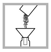
5. Add the contents of one TOC Persulfate Powder Pillow to each Acid Digestion Vial. Put a label that says "Reagent Blank" on one High Range Acid Digestion vial. Put a label that says "Sample" on a second High Range Acid Digestion vial.
