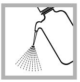
8. Use deionized water to rinse two blue Mid/High Range Indicator Ampules. Clean the ampules with a wipe. Do not touch the sides of the ampules after they are clean. Hold the ampules by the top.
