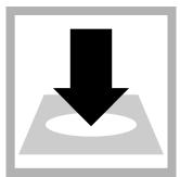
**18.** Insert the sample vial into the 16-mm cell holder.
