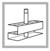
**12.** After two hours, remove the vials from the reactor. Keep the vials in an upright position at all times. Put them in a test tube rack to cool for one hour. The liquid in the blank should show a dark blue color.
