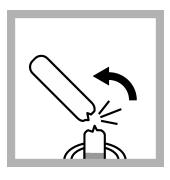
9. Put one unopened ampule into each Acid Digestion Vial. Snap the top off of the ampule when the score aligns with the top of the vial. Let the ampules drop into the vials. Do not invert or tilt the vials after the ampule is inside.
