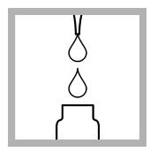
**7. Prepare the sample:** Add 0.3 mL of sample from the Erlenmeyer flask to the sample vial.
