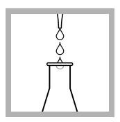
**3.** Add 0.4 mL of Buffer Solution to the Erlenmeyer flask, pH 2.0. Use pH paper to make sure that the sample pH is 2.
