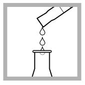
2. Add 10 mL of sample to a 50-mL Erlenmeyer flask. Put the stir bar in the Erlenmeyer flask.
