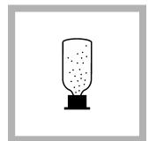
5. Hold the AccuVac Ampul with the tip down. Immediately put the cap on the tip. The cap prevents contamination from atmospheric oxygen.
