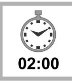
7. Start the instrument timer. A 2-minute reaction time starts. The oxygen that has degassed during aspiration dissolves again and reacts.
