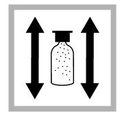
8. When the timer expires, shake the AccuVac Ampul for 30 seconds. Let all of the bubbles dissipate before the next step.
