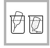
**4. Prepare the sample:** Collect at least 40 mL of sample in a 50-mL beaker. Fill the AccuVac Ampul with sample. Keep the tip immersed while the AccuVac Ampul fills completely.
