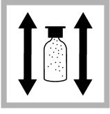
6. Shake the AccuVac Ampul for 30 seconds. A small quantity of undissolved reagent does not have an effect on the results.
