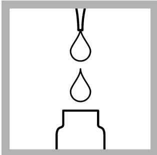
5. Use a pipet to add 2.0 mL of sample to the test vial.
