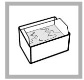
**6.** Let the vials cool to room temperature in a cool water bath, or hold under running tap water for several minutes.
