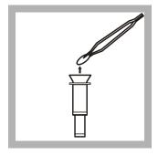
**1.** Use forceps to remove the filter from the top of the CRC.
