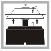
8. Open the VPD regulator to release the vacuum. Turn the pump off. Remove the VPD top and set it aside. Dispose of the used Chloride Removal Cartridges.
