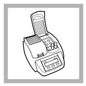
**4.** Insert the vials in the DRB200 Reactor at 150 °C. Close the cover. Digest the samples for one hour.
