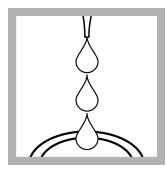
**5.** Use a pipet or dispenser to add 1.0 mL of concentrated Sulfuric Acid to both mixing cells.
