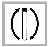
**3.** Remove the Mn III COD vial from the vacuum chamber. Put the original caps on and close tightly. Invert the vials several times to mix.
