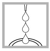
**4. Prepare the sample:** Use a pipet to add 9.0 mL of homogenized sample to a second glass mixing cell.
