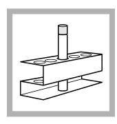
**5.** After an hour, remove the vials from the DRB200. Let the vials cool in a rack for two minutes.
