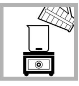
**3.** Pour the homogenized sample into a 250-mL beaker and stir slowly with a magnetic stir plate. If the sample does not have suspended solids, ignore this step.
