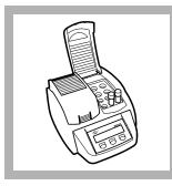
**7.** Insert the vials in the preheated DRB200 reactor. Close the cover.
