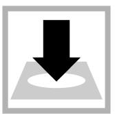
**14.** Insert the blank vial into the 16-mm cell holder.
