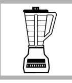
2. Measure 100 mL of sample in a blender. Blend for 30 seconds or until homogenized. If the sample does not have suspended solids, ignore this step.
