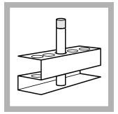
**9.** After the timer expires, let the vials cool in a test tube rack for 2 minutes. If the solution develops a colorless upper layer and a purple lower layer, invert the vials several times to mix. Use finger cots to touch hot vials.
