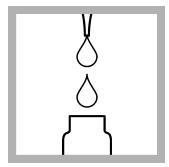
**5. Prepare the blank:** Use a pipet to add 0.5 mL of deionized water to a second test vial.
