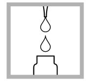
**4. Prepare the sample:** Use a pipet to add 0.5 mL of the homogenized sample to a test vial.
