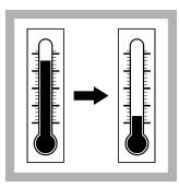
9. When the timer expires, set the reactor power to off. Let the temperature decrease for about 20 minutes to 120 °C or less.
