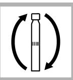
6. Hold the vial by the cap, over a sink. Invert gently several times to mix. The vial gets very hot during mixing.
