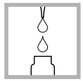
**5.** Use a pipet to add 0.3 mL of sample to the test vial.
