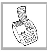
**7.** Insert the vial in the preheated DRB200 reactor. Close the lid.
