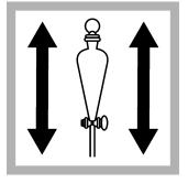
**11.** Put the stoppers on the funnels. Shake to dissolve the reagent.
