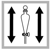
**14.** Vigorously shake each funnel for 30 seconds. Open the stopcock to vent if necessary.
