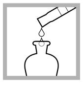
**5. Prepare the sample:** Pour the measured sample into another 500-mL separatory funnel.
