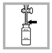
17. Drain the chloroform layers into separate sample cells (one for the blank and one for the sample). Put the stopper on the cells. The volume of chloroform extract is approximately 25 mL. The water phase in the funnel contains chloroform. Make sure to dispose of the solution properly.
