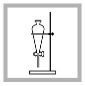
15. Remove the stoppers. Wait for the layers to separate. If there is phenol in the sample, the bottom chloroform layer will have a yellow to amber color.
