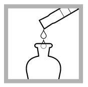
**3. Prepare the blank:** Pour the measured deionized water into a 500-mL separatory funnel.
