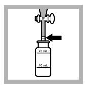
**16.** Put a cotton plug the size of a pea into the delivery tube of each funnel to remove suspended water or particles from the chloroform.
