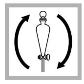
**13.** Put the stoppers on the funnels. Invert each funnel and open the stopcock to vent. Close the stopcocks, shake each funnel briefly, then invert and open the stopcock to vent.
