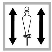
**9.** Put the stoppers on the funnels. Shake to dissolve the reagent.
