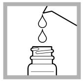
**4.** Prepare the digested sample: Fill a mixing bottle to the **25-mL mark** with the diluted sample from step 2.
