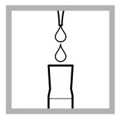
2. Select the sample size from Table 2 on page 5. Use a pipet to add the correct volume of sample into a 50-mL graduated cylinder.
