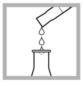
**4. Prepare the blank:** Measure 25 mL of deionized water in the graduated cylinder. Pour the water into the Erlenmeyer flask.
