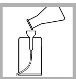
**10.** When the timer expires, pour the contents of the flask that contains the blank into the Pour-Thru Cell.
