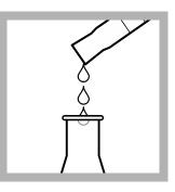
6. Prepare the sample: Measure 25 mL of sample in the graduated cylinder. Pour the sample into the second Erlenmeyer flask.
