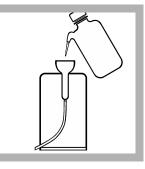
**14.** Flush the Pour-Thru Cell with at least 50-mL of deionized water immediately after use.
