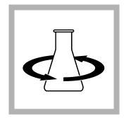
8. Swirl to mix. A yellow color forms if phosphate is in the sample. A small amount of yellow can form in the blank because of the reagent color.
