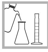
**3.** Rinse a clean plastic 125-mL Erlenmeyer flask and a 25-mL graduated cylinder with deionized water.
