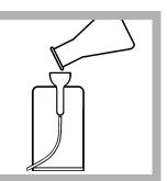
**12.** Pour the prepared sample into the Pour-Thru Cell.
