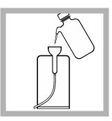
2. Flush the Pour-Thru Cell with at least 50-mL of deionized water.
