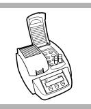
**6.** Insert the vial into the reactor. Close the reactor.
