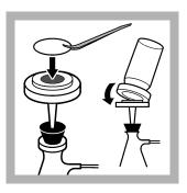
4. If the sample is turbid, set up the filtration apparatus (0.45 micron membrane filter, filter holder/funnel, filter flask, and aspirator). If the sample is not turbid, go to step 10.
