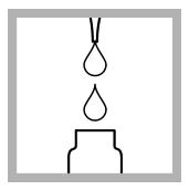
**3.** Use a pipet to add 2.0 mL of sample to the test vial.
