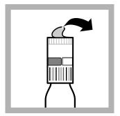
2. Carefully remove the lid from the DosiCap™ Zip cap. Remove the cap from the test vial.
