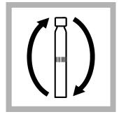
**4.** Tighten the cap on the vial and invert the vial 2–3 times.
