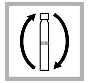
**12.** Tighten the cap on the vial and invert the vial 2–3 times.
