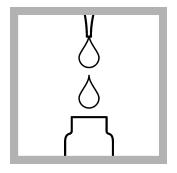
**1.** Use a pipet to add 0.5 mL of sample to the test vial.
