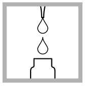
**3.** Use a pipet to add 0.5 mL of sample to the test vial.
