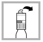
2. Carefully remove the lid from the DosiCap™ Zip cap. Remove the cap from the test vial.
