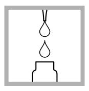
**10.** Use a pipet to add 0.2 mL of Solution B to the test vial. Immediately tighten the cap on the Solution B container.
