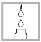
**2.** Use a pipet to add 0.2 mL of Solution B to the test vial. Immediately tighten the cap on the Solution B container.
