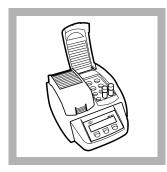
**6.** Insert the vial in the preheated DRB200 reactor. Close the lid.
