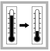
8. When the timer expires, carefully remove the vial from the reactor. Set the vial in a test tube rack. Let the temperature of the vial decrease to room temperature.
