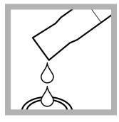
**9.** Pour 10 mL of the solution from the mixing cylinder into the sample cell.
