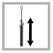
17. Immediately clean the graduated cylinder and sample cells with soapy water and a brush. Rinse with deionized water.
