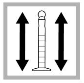
7. Put the stopper on the mixing cylinder. Shake the cylinder for 30 seconds. A white turbidity forms if potassium is in the sample.
