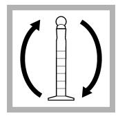
**5.** Put the stopper on the mixing cylinder. Invert the mixing cylinder several times to mix. Let the solution become clear.
