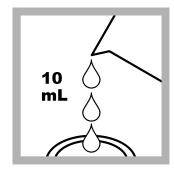
**10. Prepare the blank:** Fill a sample cell with 10 mL of fresh sample.
