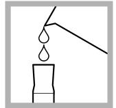
2. Prepare the sample: Fill a mixing cylinder to the 25-mL line with sample. DR 900: Use a 25-mL sample cell as an alternative to the mixing cylinder.
