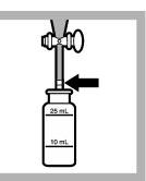
24. Insert a dry cotton plug into the outlet tube of each separatory funnel to filter the toluene and remove water or suspended particles. Identify the sample cells as blank and sample. Slowly drain the toluene from the funnels into the respective sample cells. Close the sample cells with stoppers.
