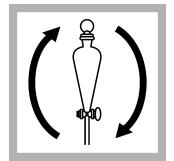
**17.** Swirl and invert each funnel, then open the stopcock to vent the funnel. Close the stopcock. Do this step two times with each funnel.
