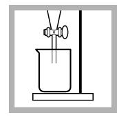
**23.** When the timer expires, remove the stopper and drain the lower water layer from each funnel and retain for disposal. Complete steps 24–29 within 5 minutes after the
