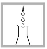
8. For non-distilled samples: Add 5.0 mL of Buffer Solution, sulfate type, pH 2.0 to each flask.
