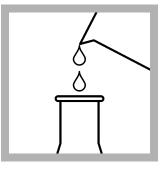
**3. Prepare the sample:** Use a graduated cylinder to add 100 mL of sample into a 500-mL Erlenmeyer flask. Put a mark on the flask to identify the flask as the sample.
