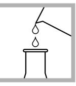
2. Prepare the blank: Use a graduated cylinder to add 100 mL of deionized water into a 500-mL Erlenmeyer flask. Put a mark on the flask to identify the flask as the blank.
