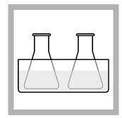
12. When the timer expires, remove both flasks from the hot plate. Decrease the temperature of the flasks to approximately 25 °C (77 °F) in a water bath.
