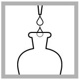
14. Use a calibrated 1.0-mL plastic dropper to add 2.0 mL of 12 N Potassium Hydroxide Standard Solution to each funnel. Put the stopper on the funnels.
