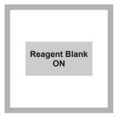
2. Set the reagent blank option to on to automatically subtract the reagent blank value from the sample results.
