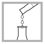
**7.** Pour the contents of the 50-mL cylinder back into the original flask.
