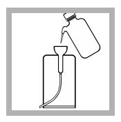
**21.** Flush the Pour-Thru Cell with at least 50-mL of deionized water immediately after use.
