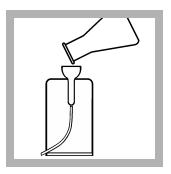
**15.** When the timer expires, pour the contents of one flask into the Pour-Thru Cell.
