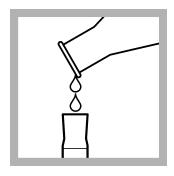
**5.** Fill a clean 50-mL plastic graduated cylinder with sample from one of the flasks. Then discard the contents of the cylinder. Do this procedure three times.
