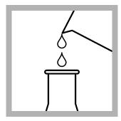
**4.** Fill two clean 250-mL Erlenmeyer flasks to overflowing with sample.
