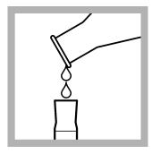
**6.** Fill the rinsed cylinder to the 50-mL mark with sample from the same flask. Discard any remaining sample in the flask.
