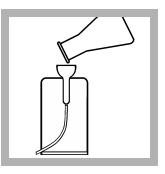
**19.** Wait at least 15 seconds, then pour the contents of the second flask into the Pour-Thru Cell.
