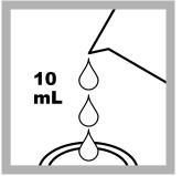
2. Prepare the blank: Fill a sample cell with 10 mL of sample.
