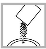
**10.** After the timer expires, add the contents of one Amino Acid F Reagent powder pillow to the prepared sample cell.
