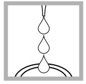
**4.** Add 14 drops of Molybdate 3 reagent solution to each cell.
