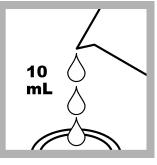
**10. Prepare the blank:** Fill a second sample cell with 10 mL of the original sample.
