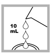
Prepare the blank: Fill a second sample cell with 10 mL of sample.
