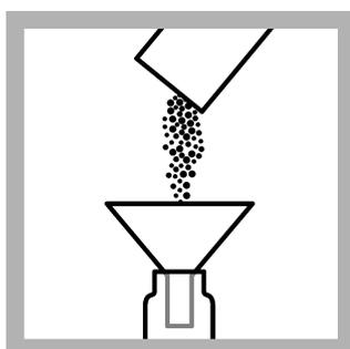
6. Write "control" on one Test 'N Tube vial. Then, open one ToxTrak Reagent Powder Pillow and add the contents to the empty tube.
