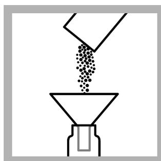
7. For each sample or dilution, write the sample number on each Test 'N Tube vial. Then, open one ToxTrak Reagent Powder Pillow and add the contents to the empty sample vial.
