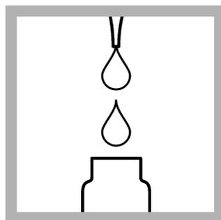
9. Add 5.0 mL of sample (or dilution) to each sample vial. Refer to [Interpreting results](#) on page 5 to find the approximate threshold level of toxicity for a sample.
