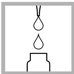
2. **Prepare the blank:** Fill an empty Test 'N Tube vial to the top of the label with deionized water.
