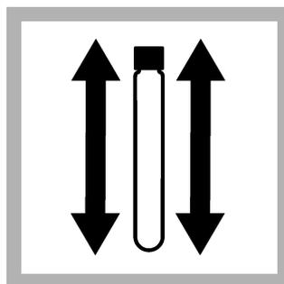
11. Close the tube and shake to mix. Shake to fully oxygenate the samples, so that the oxygen concentration does not affect the respiration rate.
