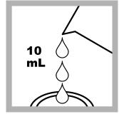
**4. Prepare the sample:** Put a mark on a round sample cell to identify the cell as the sample. Fill the sample cell with 10 mL of sample.
