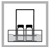
**20.** When the timer expires, remove the assembly from the cooling bath. Remove the sample cells from the assembly rack. Make sure that the temperature of the sample is 15–25 °C.
