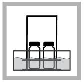
**18.** Replace the water in the cooling bath with new cold tap water. Put the assembly with the cells into the cooling bath. If necessary, use ice to decrease the temperature of the tap water.
