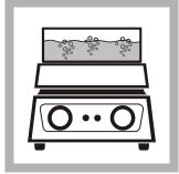
2. Add 500 mL of water to an evaporating dish to prepare a hot water bath. Put the dish on a hot plate and set the heater to high.
