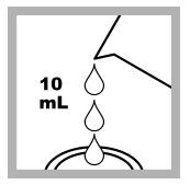
5. Prepare the blank: Put a mark on a second round sample cell to identify the cell as the blank. Fill the sample cell with 10 mL of deionized water.
