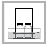
13. When the timer expires, remove the assembly from the hot water bath. Put the assembly in the cooling bath.
