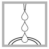
**17.** Use a TenSette Pipet to add 1 mL of THM Plus Reagent 3 to each sample cell. The sample and the blank will become warm.
