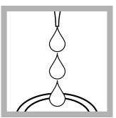
8. With a TenSette<sup>®</sup> Pipet, add 3 mL of THM Plus Reagent 2 to each sample cell. Prevent agitation of the sample when the reagent is dispensed.
