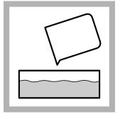
**3.** Add 500 mL of cold tap water (18 to 25 °C) to a second evaporating dish. Keep the temperature in this range.
