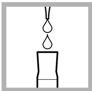
**6. Prepared sample:** Use a plastic dropper to add 0.5 mL of cyclohexanone to the solution in the mixing cylinder.
