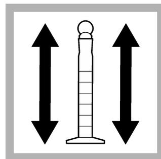
**8.** During the reaction period, close the mixing cylinder and vigorously shake the prepared sample. The sample becomes reddish-orange, brown or blue, depending on the zinc concentration.
