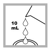
**6. Prepare the blank:** Fill a sample cell with 10 mL of unreacted sample.
