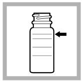
2. Prepare the sample: Fill a marked bottle to the 25-mL line with sample. For instruments that measure with a 25-mL sample cell, prepare the sample in the sample cell.
