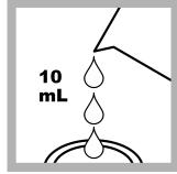
**10.** When the timer expires, fill a second sample cell with 10 mL of prepared sample from the mixing bottle.
