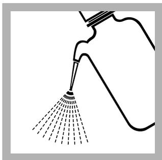
1. Rinse the probe with deionized water. Dry the probe with a lint-free cloth.
