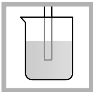
2. **Laboratory test:** Put the probe in a beaker that contains the solution. Do not let the probe touch the stir bar, bottom or sides of the container. Remove the air bubbles from under the probe tip. Stir the sample at a slow to moderate rate.
