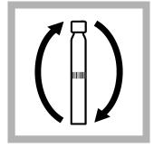
**4.** Tighten the cap on the vial and invert the vial 2–3 times. Carefully rotate the vial to remove air bubbles. Do not shake.
