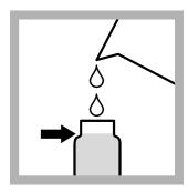
**3.** Fill the sample vial with sample to the throat of the vial.
