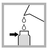
**3.** Complete this procedure within 1 minute: Fill the sample vial with sample to the throat of the vial.
