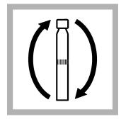
**5.** Tighten the cap on the vial and invert the vial 2–3 times. Carefully rotate the vial to remove air bubbles. Do not shake.
