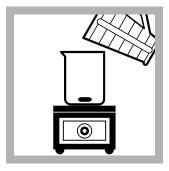
3. Pour the homogenized sample into a 250-mL beaker and stir slowly with a magnetic stir plate. If the sample does not have suspended solids, ignore this step.
