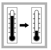
**11.** Put the vial in a test tube rack. Let the temperature of the vial decrease to room temperature.
