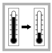
9. When the timer expires, set the reactor power to off. Let the temperature decrease for about 20 minutes to 120 °C or less
