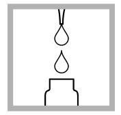
**5.** Use a pipet to add 2.0 mL of sample to the test vial.
