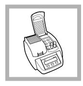
7. Insert the vial in the preheated DRB200 reactor. Close the lid.
