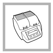
**1.** Set the DRB200 reactor power to on. Set the temperature to 150 °C.
