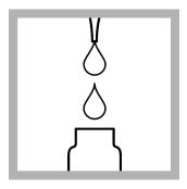
**1.** Use a pipet to add 2.0 mL of sample to the test vial.
