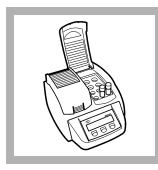
**3.** Insert the reaction tube in the preheated DRB200 reactor. Close the lid.
