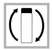
**7.** Tighten the cap on the reaction tube and invert until completely mixed.
