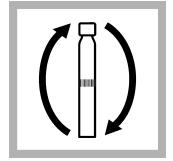
**13.** Quickly tighten the cap on the vial and invert until completely mixed.
