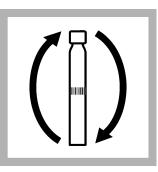
**10.** Quickly tighten the cap on the vial and invert until completely mixed. Immediately continue to the next step.
