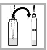
**8.** Use a pipet to add 0.5 mL of the digested sample from the 20-mm reaction tube into a test vial 1 (red label).
