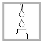
**9.** Use a pipet to add 0.2 mL of Solution D to the test vial.
