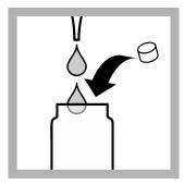
2. Add 1.3 mL of sample, 1.3 mL of Solution A and 1 Reagent B tablet in quick succession to a dry 20-mm reaction tube. Close the reaction tube immediately. Do not invert.
