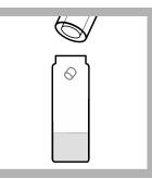
**6.** When cool, add 1 Micro Cap C to the reaction tube.
