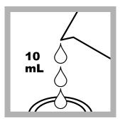
**6. Prepare the sample:** Fill a second sample cell with 10 mL of sample.
