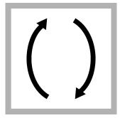
8. Put the stopper on the prepared sample cell. Invert the sample cell several times to mix. A pink color shows if chlorine is present. Go to the next step immediately.
