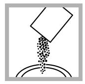
**7.** Add the contents of one DPD Free Chlorine Powder Pillow for 25-mL sample to the prepared sample cell.
