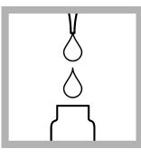
**10.** Use a pipet to add 0.2 mL of Solution B to each vial. Immediately tighten the cap on the Solution B container.
