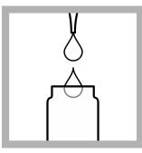
**3. Prepare the blank:** Use a pipet to add 3.5 mL of deionized water into one test vial.
