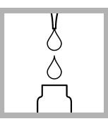
**3.** Use a pipet to add 0.2 mL of Solution B to each vial. Immediately tighten the cap on the Solution B container.
