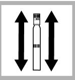
**6.** Shake each vial 2–3 times to dissolve the reagent in the cap. Look through the open end of the DosiCap to make sure that the reagent has dissolved.
