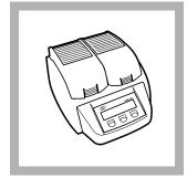
**1.** Set the DRB200 reactor power to on. Set the temperature to 100 °C.
