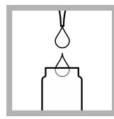
**1. Prepare the blank:** Use a pipet to add 3.5 mL of deionized water into one test vial.
