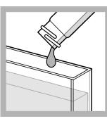
**8.** Pour the blank into the sample cell.
