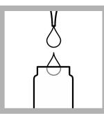
**2. Prepare the sample:** Use a pipet to add 3.5 mL of sample into the other test vial.
