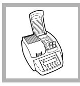
**7.** Insert the vials in the preheated DRB200 reactor. Close the lid.
