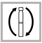
**12.** Tighten the cap on the vials and invert the vials 2–3 times.
