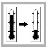
**9.** When the timer expires, carefully remove the vials from the reactor. Set the vials in a test tube rack. Let the temperature of the vials decrease to room temperature.
