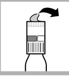
2. Carefully remove the lids from the DosiCap<sup>™</sup> Zip caps. Remove the caps from the test vials.
