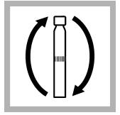
**5.** Tighten the cap on the vials and invert the vials 2–3 times.
