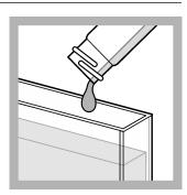
**20.** Pour the digested sample into a second sample cell.
