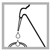
3. If the sample volume is less than 25-mL, add deionized water to the 25-mL line.
