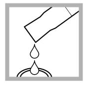
**10.** Pour 10 mL of the solution from the mixing cylinder into the sample cell.
