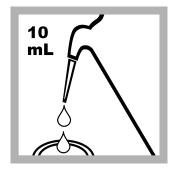
**12.** If the sample volume is less than 10-mL, add deionized water to the 10-mL line.
