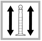
**8.** Put the stopper on the mixing cylinder. Shake the cylinder for 30 seconds. A white turbidity forms if potassium is in the sample.
