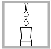
2. Prepare the sample: Add the sample volume that is specified for the test range to a 25-mL mixing cylinder:
