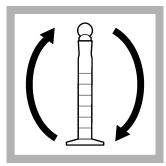
**6.** Put the stopper on the mixing cylinder. Invert the mixing cylinder several times to mix. Let the solution become clear.
