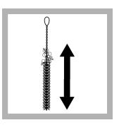
**19.** Immediately clean the graduated cylinder and sample cells with soapy water and a brush. Rinse with deionized water.
