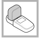
**15.** Install the instrument cap over the cell holder.
