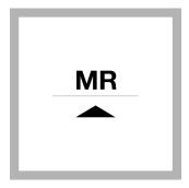
1. Set the instrument to mid-range (MR). For DR300, push the up arrow button. For PCII, push the menu button, checkmark button, then the menu button again.
