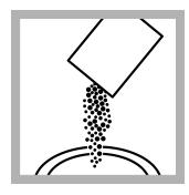
**9.** Add one 25-mL DPD Free Chlorine Reagent Powder Pillow or one 25-mL DPD Total Chlorine Reagent Powder Pillow to the second sample cell.
