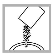
**11.** Add the contents of one PhosVer 3 Phosphate Reagent Powder Pillow to both the blank and the prepared sample.
