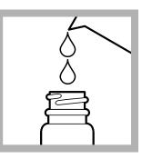
**3. Prepare the digested sample:** Pour 25-mL of the diluted sample from step 1 into a mixing bottle.
