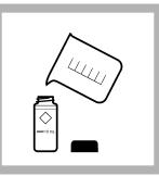
**10. Prepare the sample:** Fill a second sample cell to the 10-mL mark with the digested sample.
