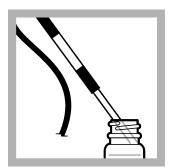
**9.** When the timer expires, turn off the UV lamp. Remove the UV lamp from the sample.
