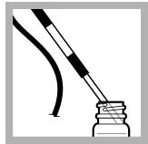
**7.** Put the ultraviolet lamp into the mixing bottle. Turn on the UV lamp.
