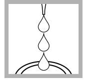
**9.** Add 0.5 mL of Phenol Red Indicator Solution to the blank.
