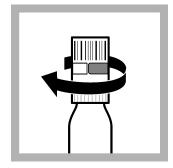
**3.** Turn the DosiCap Zip over so that the reagent side goes on the test vial. Tighten the cap on the vial.
