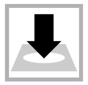
**11.** Insert the vial into the cell holder. DR1900 only: Push **READ**. Results show in CN<sup>-</sup>.
