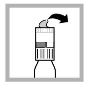
1. Carefully remove the lid from the DosiCap™ Zip cap. Remove the cap from the test vial.
