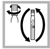
**6.** Tighten the cap on the vial and invert the vial 2–3 times.
