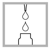
**5.** Use a pipet to add 1.0 mL of Solution A to the test vial.
