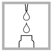
2. Use a pipet to add 1.0 mL of sample to the test vial. Immediately continue to the next step.
