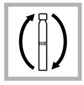
2. Tighten the cap on the vial and invert the vial 2–3 times.
