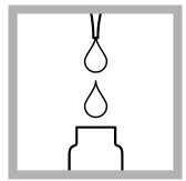
**4.** Use a pipet to add 3.0 mL of sample to the test vial.
