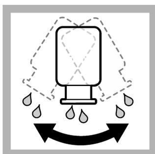
6. Discard the solution from the sample cell. Shake to remove excess solution from the sample cell.
