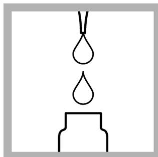
3. Use the dropping bottle to add 8 drops of the FerroZine Reagent Solution to the reaction tube.
