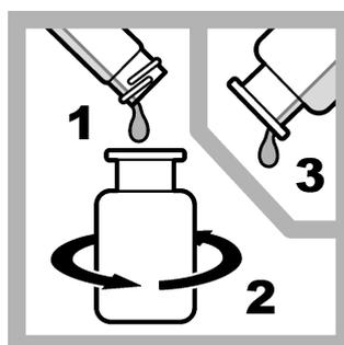
7. Rinse the sample cell with a small portion of the digested sample.
