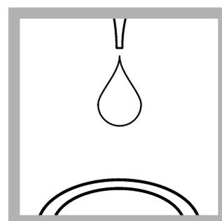
12. Use the dropping bottle to add 8 more drops of the FerroZine Reagent Solution to the sample cell.
