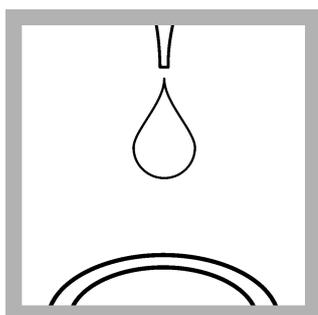
6. Use the dropping bottle to add 8 drops of the FerroZine Reagent Solution to the sample cell.
