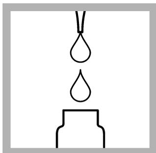
2. **Prepare the sample:** Pour 12 mL of sample into a 20-mm reaction tube.
