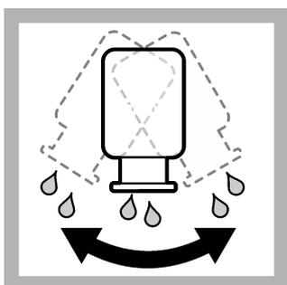
21. Discard the solution from the sample cell. Shake to remove excess solution from the sample cell.
