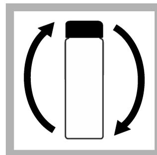
4. Tighten the cap on the reaction tube and invert to mix.
