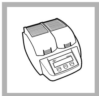
1. Set the DRB200 reactor power to on. Set the temperature to 135 °C.
