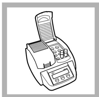
5. Insert the reaction tube in the preheated DRB200 reactor. Close the lid.
