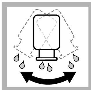
19. Discard the solution from the sample cell. Shake to remove excess solution from the sample cell.
