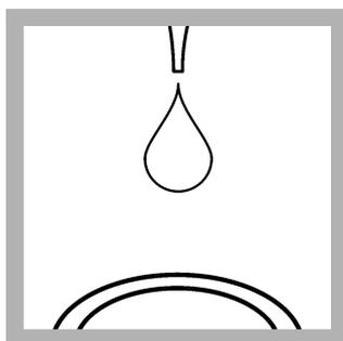
2. Add 10 mL of deionized water to the sample cell. The same sample cell must be used to measure the color of the reagent and the sample.
