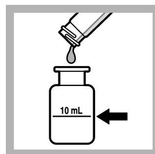
8. Pour 10 mL of the digested sample into the same sample cell.
