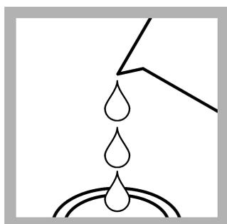
**2. Prepare the blank:** Fill a sample cell to the 10-mL mark with sample.
