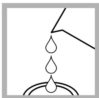
**6. Prepare the sample:** Fill a second sample cell to the 10-mL mark with sample.
