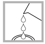
**2. Prepare the blank:** Fill a sample cell to the 10-mL mark with sample.
