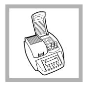
7. Insert the vial in the preheated DRB200 reactor. Close the lid.
