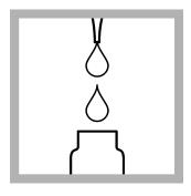
**1.** Use a pipet to add 4.0 mL of Solution A to the test vial.
