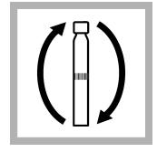
**9.** Tighten the cap on the vial and invert the vial 2–3 times.
