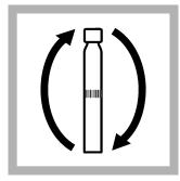
**2.** Tighten the cap on the vial and invert until completely mixed.
