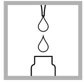
**14.** Use a pipet to add 0.2 mL of Solution B to the test vial.
