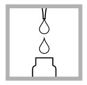
**8.** Use a pipet to add 0.2 mL of sample to the test vial.
