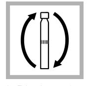
**15.** Tighten the cap on the vial and invert the vial 2–3 times.
