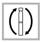
**9.** Tighten the cap on the vial and invert the vial 2–3 times.
