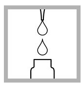
**3.** Use a pipet to add 1.5 mL of Solution A to the test vial.
