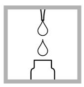
**2.** Use a pipet to add 1.5 mL of sample to the test vial.
