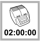
**7.** Keep the vial in the reactor for 2 hours.
