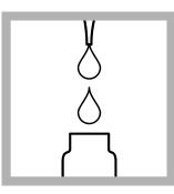
2. Use a pipet to add 1.8 mL of sample to the test vial.
