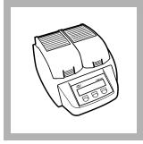
**5.** Set the DRB200 reactor power to on. Set the temperature to 150 °C (302 °F).
