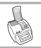
**6.** Insert the vial in the preheated DRB200 reactor. Close the lid.
